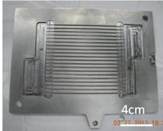
Figure III. 9 Interconnector with serpentine flow pattern
