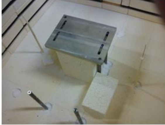
Figure III. 15 current connectors and thermocouples fixed in bottom plate
