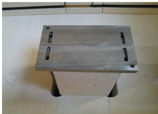
Figure III. 12 Gas module separated by brick from base plate
