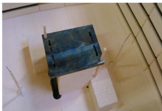
Figure III. 13 Gas module aligned with ceramic tubes
