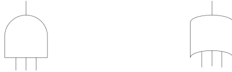
Figure 2.1: Example of two logic gates: AND gate on the left, OR gate on the right
