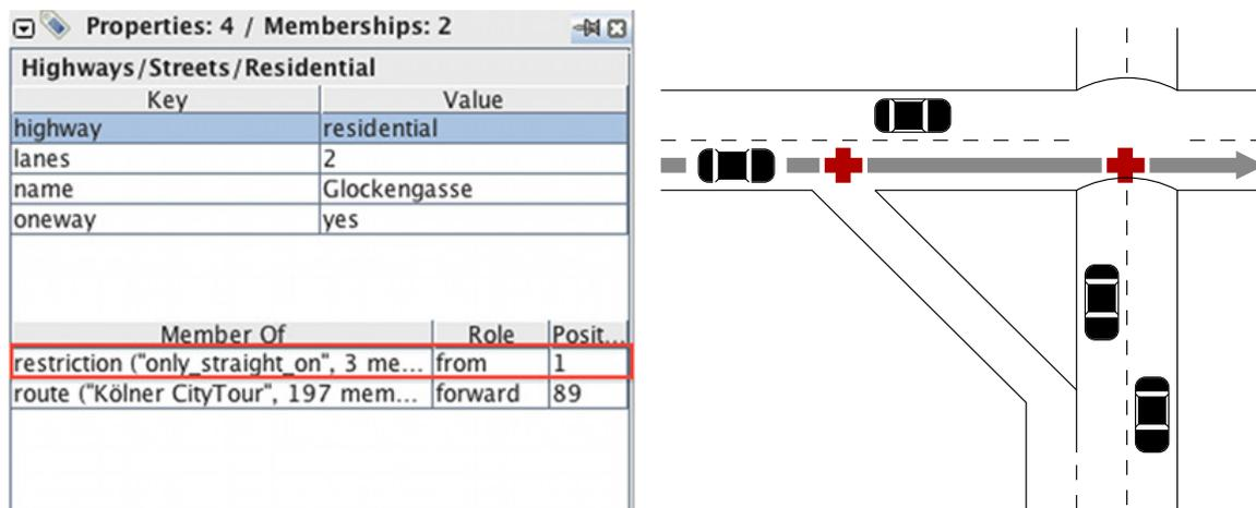
Figure 3.6: Example of continuous restriction enforcement in OpenStreetMap
