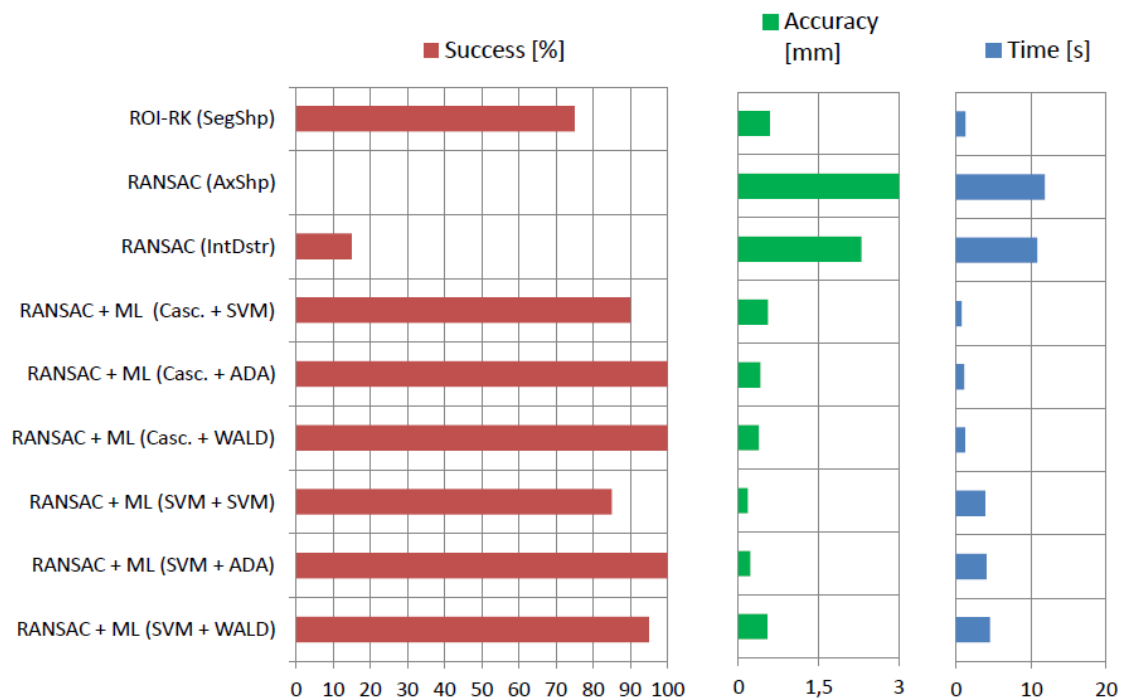
Fig. 5-8 Results of tool localization on the PVA cryogel phantom. The first column is the failure rate for all the methods expressed as a percentage; the second column is the axis accuracy in mm; the third column is the calculation time for each method.
