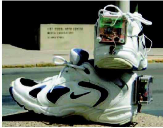
Figure 2.15: Piezoelectric-powered shoes with mounted electronics[13].
