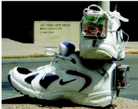
Figure 2.15: Piezoelectric-powered shoes with mounted electronics[13].
