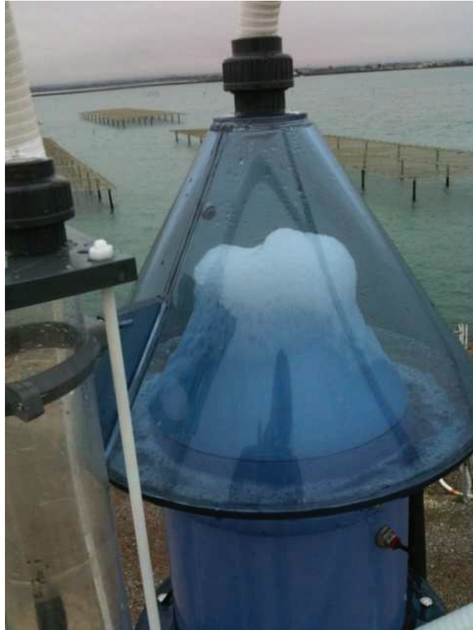
Figure 2.3: Bicone for foam harvesting at the top of the column.
