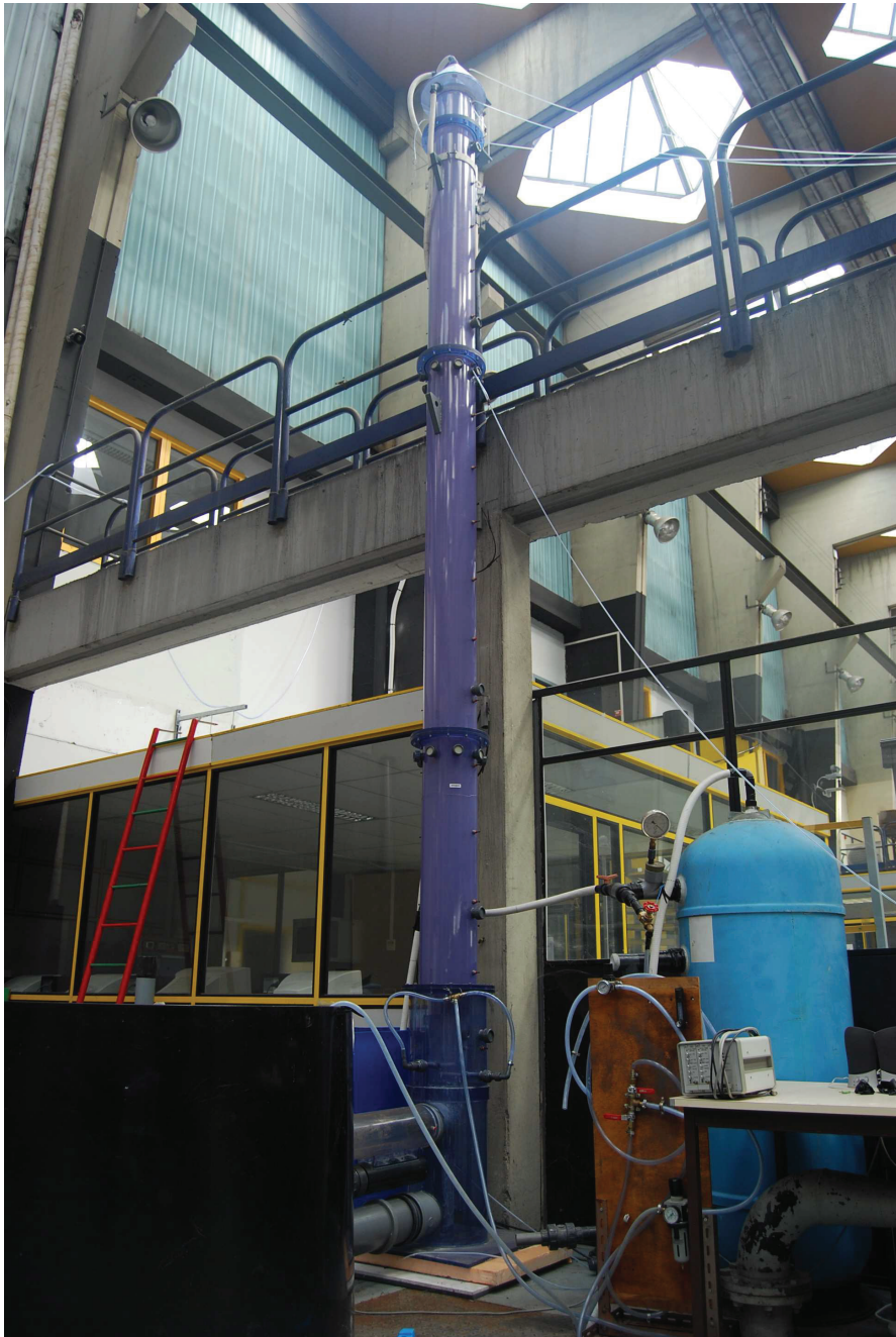
Figure 2.2: Bubble column of the LMFA.
