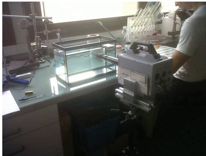
Figure 2.5: Experimental setup for the measurement of bubble diameters generated by wood and ceramic diffusers.
