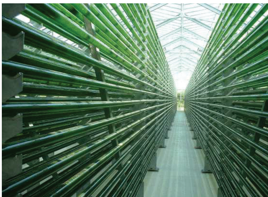
Figure 1.1: Horizontal pipe photobioreactor.
