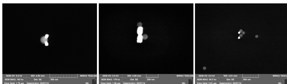
(a) Single particle on a bigger than expected gap (b) Two particles captured on a bridged "dimer" (c) Three particles on a dimer and two non-specifically adsorbed on surrounding silica
