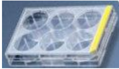
Figure 8-1 Tissue culture test plate with surface area of 8.96 \text{ cm}^2 for each well used in this study.
