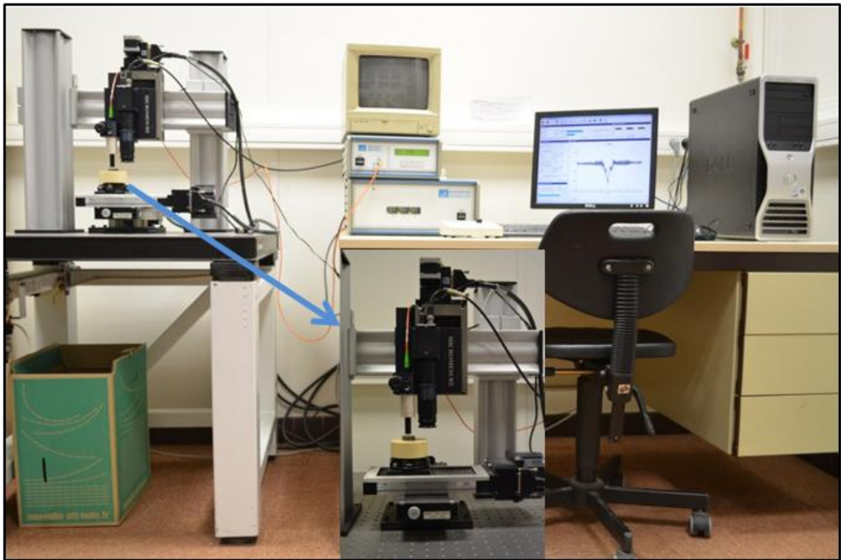
Figure 3-9 3-D optical profilometry used in this work.
