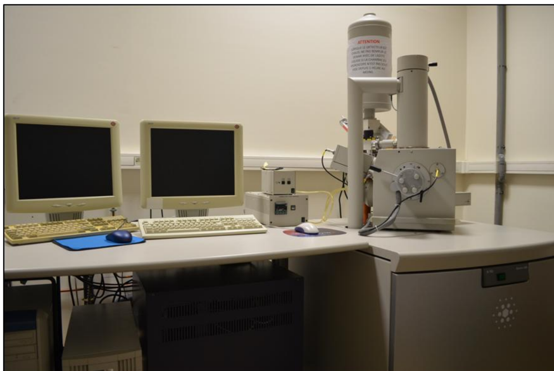
Figure 3-12 Setup of SEM coupled with EDS.
