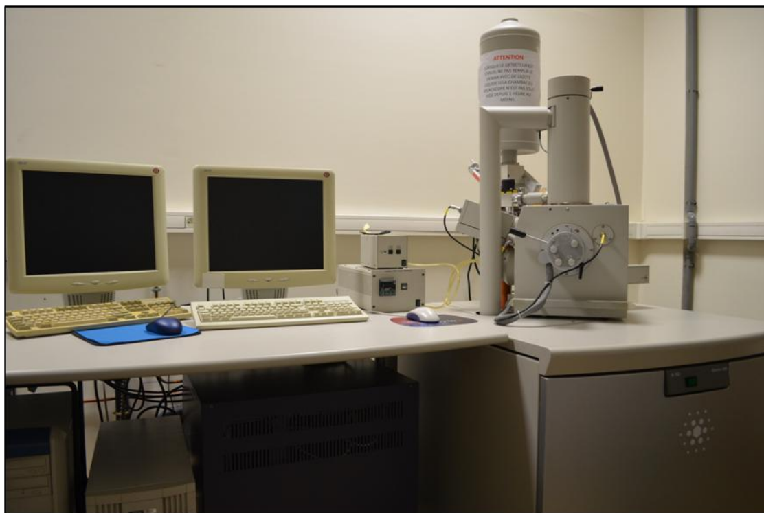
Figure 3-12 Setup of SEM coupled with EDS.
