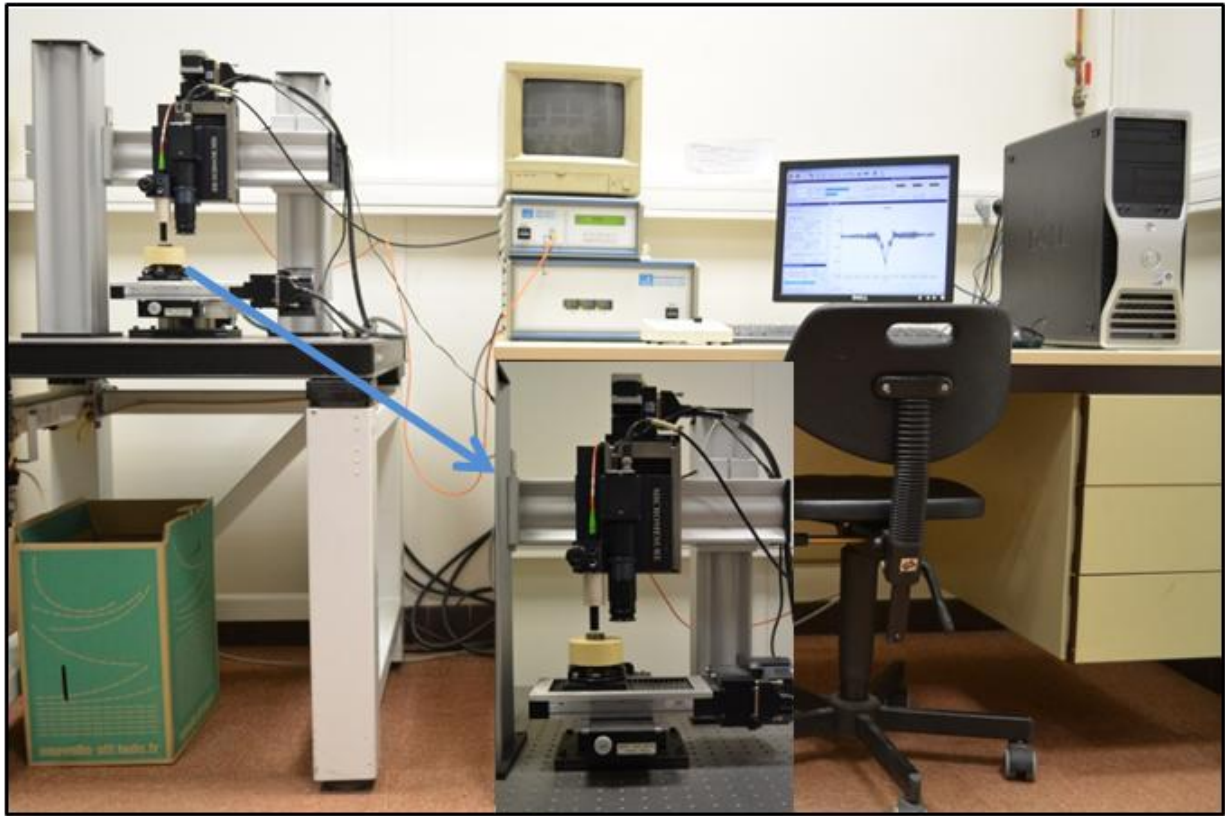
Figure 3-9 3-D optical profilometry used in this work.
