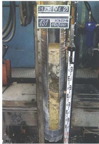
Figure 2.6: Typical core sample from conventional lines (obtained from Duong et al., 2014b ).
