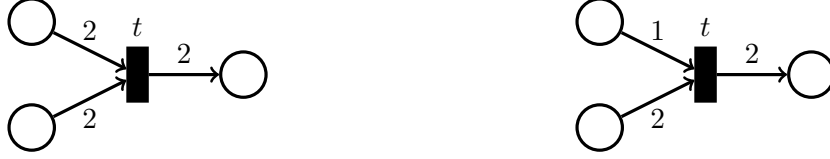
Figure 3.5: The transition t on the left is normalized. On the right, t is not normalized.
