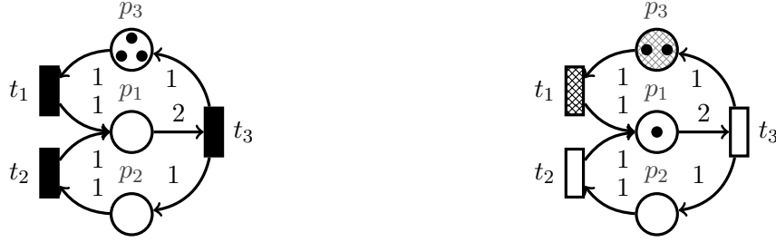
Figure 5.6: Two well-formed FA systems with minimal T-semiflow (1, 1, 1) . Relatively to this T-semiflow, the transient FA system on the right, obtained by firing the sequence t_1 in the system on the left, does not contain any enabled ready transition (white transitions) since the only enabled one is t_1 , which is frozen (dashed transition). Consequently, this transient system is blocking.
