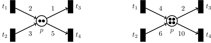
Figure 3.1: The marked place on the left is scaled by 2, yielding the place on the right.
