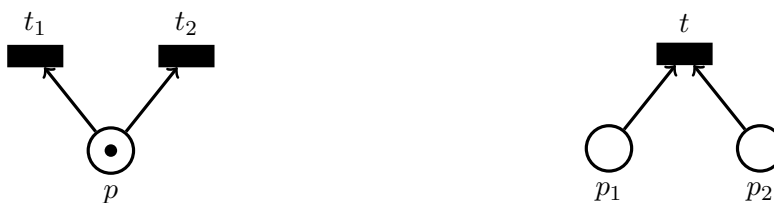
Figure 2.7: On the left, transitions t_1 and t_2 are in conflict and p is a choice-place. On the right, t is a join-transition, modeling a synchronization of its input places p_1 and p_2 .
