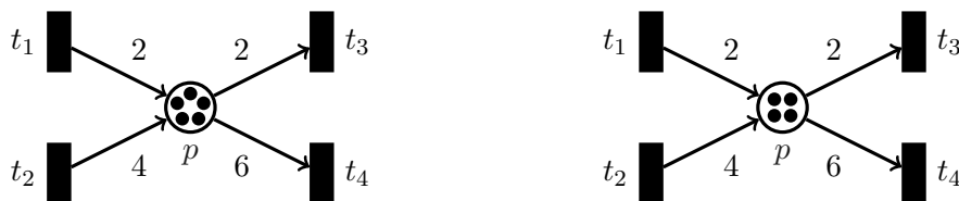
Figure 3.8: The \gcd of the places equals 2. The marking on the left does not fulfill the useful tokens condition, hence it can be reduced while preserving the language. On the right, the place fulfills the condition and induces the same language.
