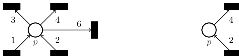
Figure 5.24: On the left, gcd_p = 1 , max_p = 6 and max_p - gcd_p = 5 . In the T-subsystem on the right, gcd_p = 2 , max_p = 4 and max_p - gcd_p = 2 .
