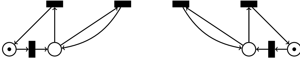
Figure 5.18: The two P-components of the well-behaved Equal-Conflict system of Figure 5.17 are well-behaved and reversible.
