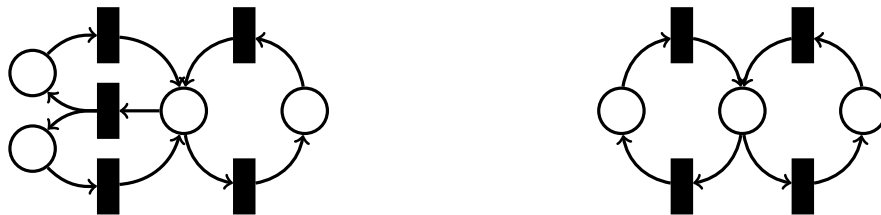
Figure 2.14: On the left, a Join-Free net that is not an S-net. The net on the right is an S-net.
