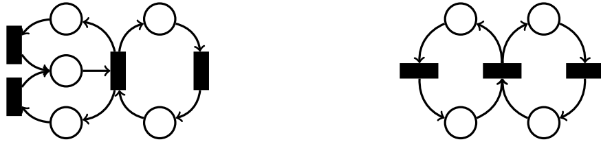
Figure 2.13: On the left, a Choice-Free net that is not a T-net. The net on the right is a T-net.
