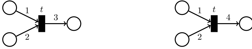
Figure 3.3: On the left, a token-conservative transition t . On the right, a non token-conservative transition t .
