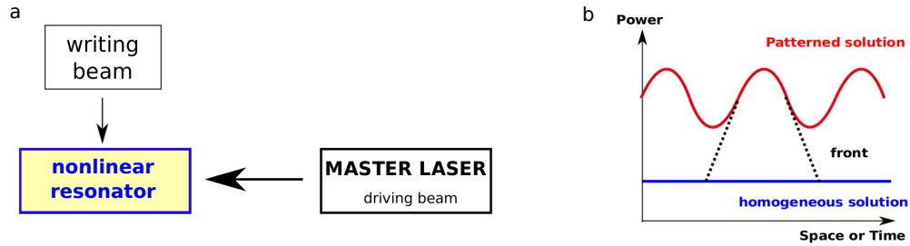
Figure 1.14: a) Schematic of experiments for CS implementation. The nonlinear resonator can be either the transverse section of a VCSEL for spatial localization of light or a fiber laser cavity for temporal localization. The space/time patterned state shown in b) is induced by coherent injection from an external Master beam. The writing beam creates a front connecting the homogeneous stable background with the higher intensity solution.
