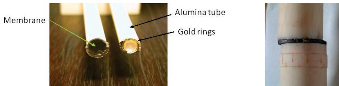
Figure 41 Membrane surface on the alumina tube (left), and membrane edge between the two alumina tubes
