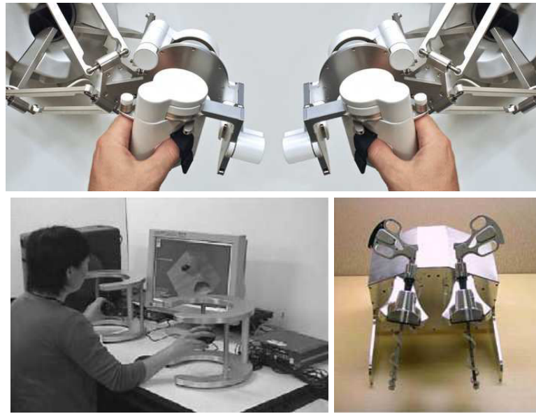
Figure 2.4 – Examples of single-point bimanual haptic interfaces with grip-force interfaces: sigma.7 (Force Dimension), SPIDAR-G&G [Murayama et al., 2004] and bimanual surgical interface [Waldron and Tollon, 2003].
