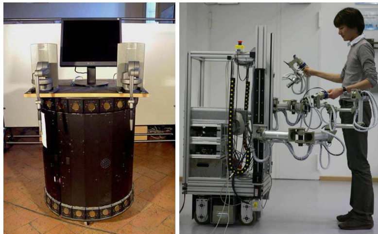
Figure 2.5 – Examples of single-point mobile bimanual haptic interfaces: Mobile Haptic Grasper [Formaglio et al., 2006] and VISHARD7-based mobile haptic interface [Peer and Buss, 2008].
