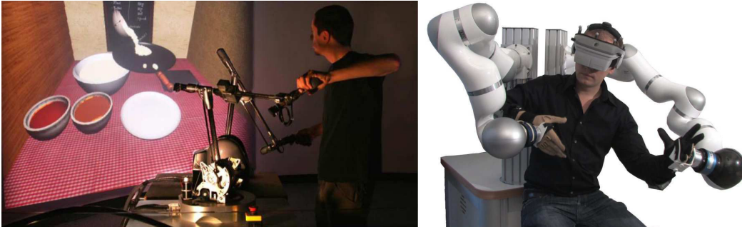
Figure 2.3 – Examples of single-point bimanual haptic interfaces: Virtuoso 6D [Cirio et al., 2011] and robot arm-based interface from DLR [Hulin et al., 2008].
