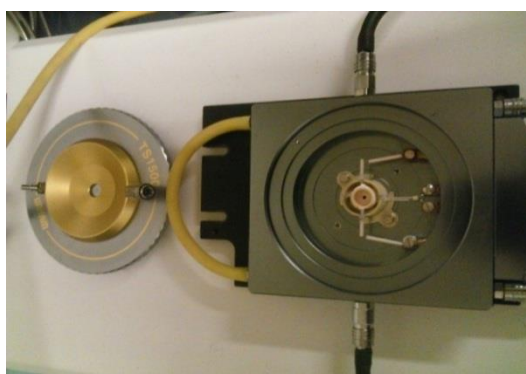
Figure II.41 : Cellule chauffante Raman in-situ
