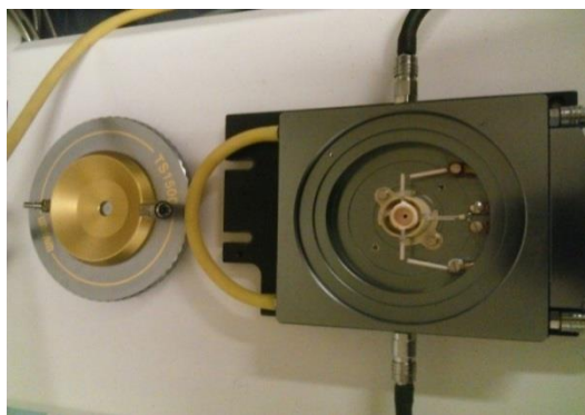
Figure II.41 : Cellule chauffante Raman in-situ
