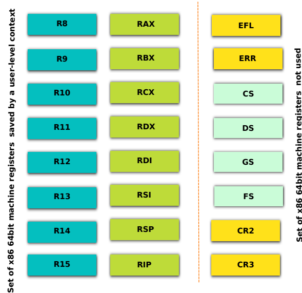
Figure 6.3: Set of registers that constitute the CPU user-context.
