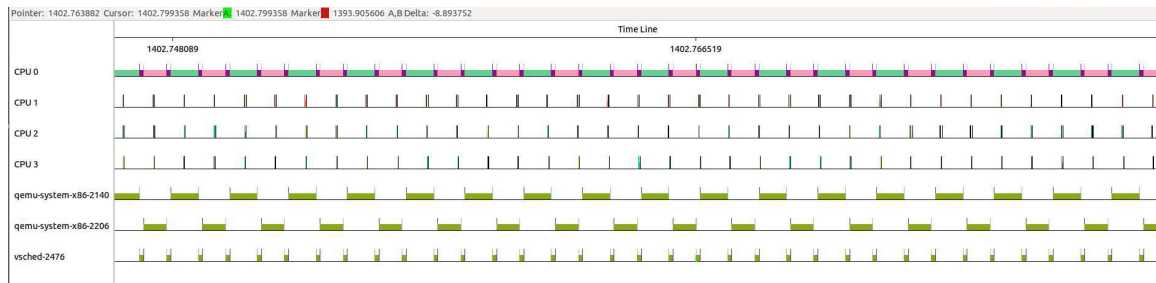
Figure 4.11: Scheduling of virtual machines using the periodic resource model. The CPU was allocated in fair-share fashion to both virtual machines.
