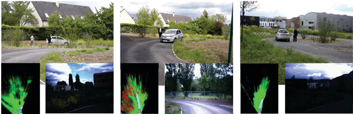
Figure 5.20 - The autonomous vehicle enabled to perform sharp curves in presence of partial occlusions.
