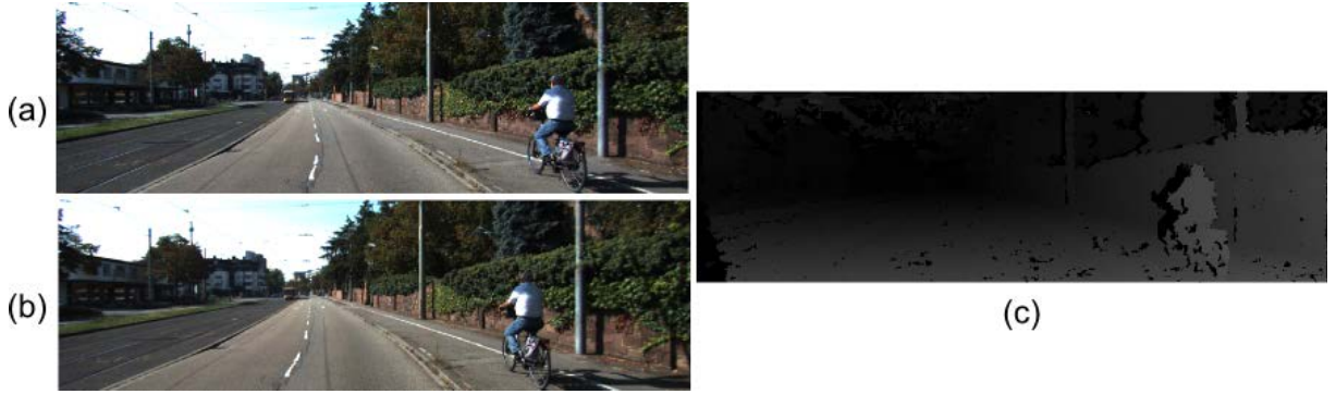
Figure 3.11 - The disparity map result applying SGBM algorithm. (a) Left image (b) Right image (c) Disparity result applying SGBM algorithm.
