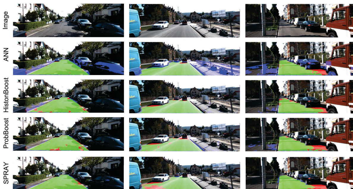
Figure 3.20 - The result process for Urban Unmarked (UU) in the perspective space. The rows present the original image, followed by ANN, HistonBoost and ProbBoost results. Green color represents True Positive, red one represents False Negative and blue defines True Negative.
