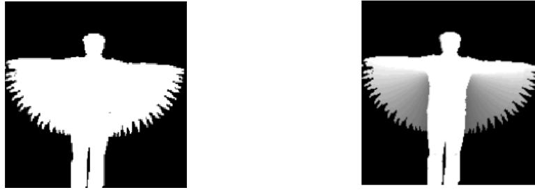
Figure 2.6: MEI (left) and MHI (right) of a person raising both hands. This figure is reproduced from [Bobick and Davis, 2001].
