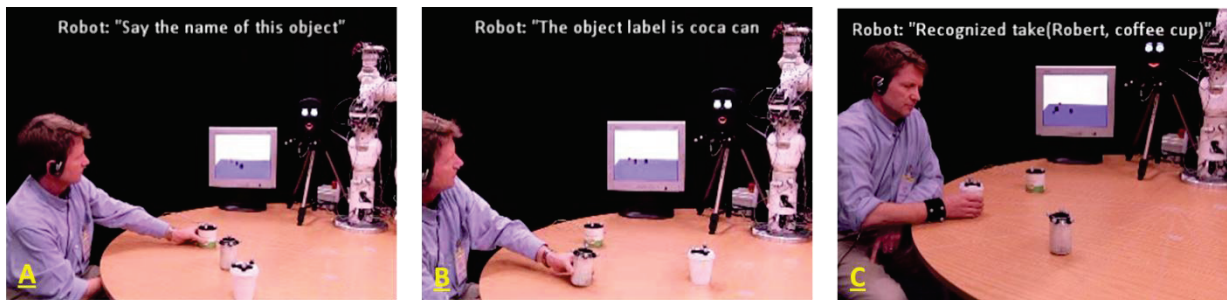
Figure 19: Visual/name binding (A, B) and use of those bindings to proceed to action learning and recognition (C) on the BERT2 platform in Bristol.
