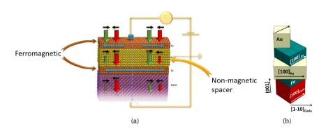
Figure II.8: (a) MagnetoResistance (GMR) device. The BEEM current depends on alignment of the ferromagnetic electrodes, because of the different transmittance for parallel or anti-parallel alignment. (b) Structure of the Fe/Au/Fe/GaAs spinvalve studied by M. Hervé et al. [25, 26]. The top film of gold is used to avoid oxydation of the iron electrode.
