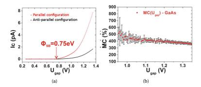
Figure II.9: (a) Room temperature Ballistic Electron Magnetic Spectroscopy perform on the Fe/Au/Fe/GaAs spinvalve, by M. Hervé *et al.*[25] and (b) resulting magneto-current. The MC seems to increase near the Schottky barrier.
