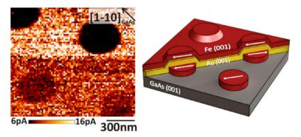
Figure II.2: Image of a buried structure (Fe(1nm)/Au(6nm)/Fe(1nm)/GaAs(001)) made using the BEEM imaging mode ( $U_{gap} = 1.5 \text{ V}$ ), from Ref. [24]. The dark regions are low current areas, while bright regions are high current area.
