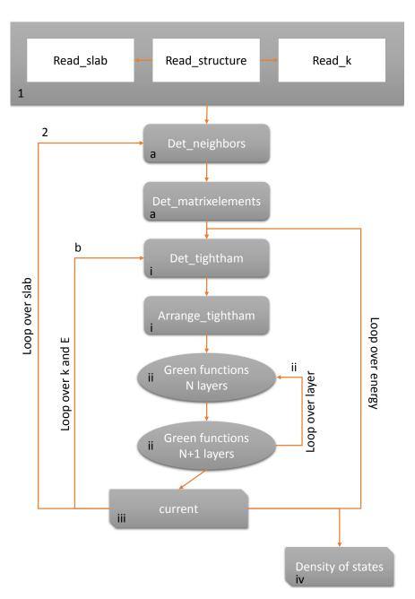
Figure IV.1: Flow chart of BEEM v3.0.
