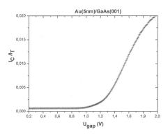
Figure II.3: Ballistic Electron Emission Spectroscopy performed on Au(5nm)/GaAs(001). The BEEM current  $I_B(U_{gap})$  starts to increase above a given threshold: the Schottky barrier. In this mode, the position xy of the tip remains constant, as well as the tunneling current through a feedback loop which varies the altitude of the tip with respect to the surface.
