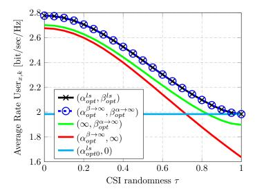
Figure 4.4: Average user rate vs. CSI quality for adaptive precoder weights  $(N=160,\,K=40,\,\varepsilon=0.7,\,P=10\mathrm{dB}).$
