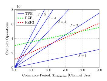
Figure 3.1: Total number of arithmetic operations of RZF precoding and TPE precoding (with different J) for K = 100 users and M = 500.
