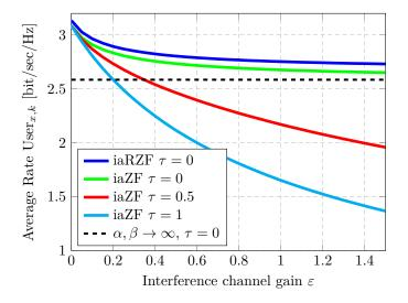
Figure 4.6: Average user rate vs. interference channel gain  $\varepsilon$  ( $N=160,\,K=40,\,\alpha=\infty,\,\beta=\beta_{opt}^{\alpha\to\infty},\,P=10{\rm dB}$ ).
