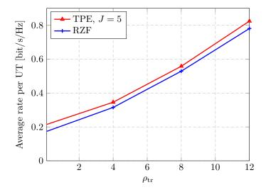
Figure 3.11: Comparison between RZF precoding and TPE precoding for a varying effective training SNR  $\rho_{\rm tr}$ .
