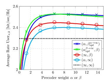
Figure 4.3: Average user rate vs. precoder weight; DE: Lines, MC: Markers  $(N=160,\,K=40,\,\tau=0.4,\,\varepsilon=0.7,\,P=10\mathrm{dB}).$
