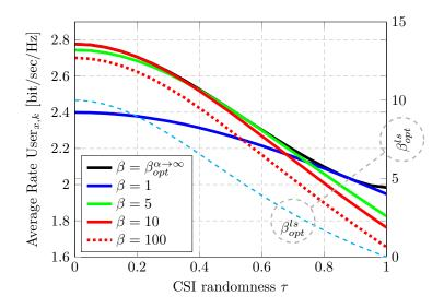
Figure 4.5: Average user rate vs. CSI quality for constant precoder weights ( $N=160,\,K=40,\,\varepsilon=0.7,\,\alpha=\alpha_{opt}^{\beta\to\infty},\,P=10{\rm dB}$ ).
