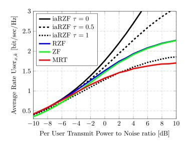
Figure 4.2: Average user rate vs. transmit power to noise ratio  $(N=160, K=40, \varepsilon=0.7, \rho_1=\rho_2=\rho)$ .
