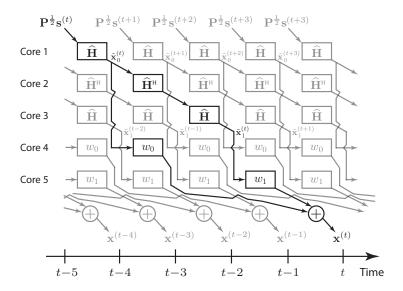
Figure 3.2: Illustration of a simple pipelined implementation of the proposed TPE precoding with J=2, which removes the delays caused by precomputing the precoding matrix. Each block performs a simple matrix-vector multiplication, which enables highly efficient hardware implementation and J can be increased by simply adding additional cores.
