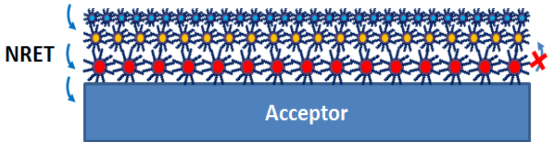
Figure 3.9: Schematic of a multilayer channel of quantum dots. Energy is transferred from the top layer all the way the acceptor substrate.
