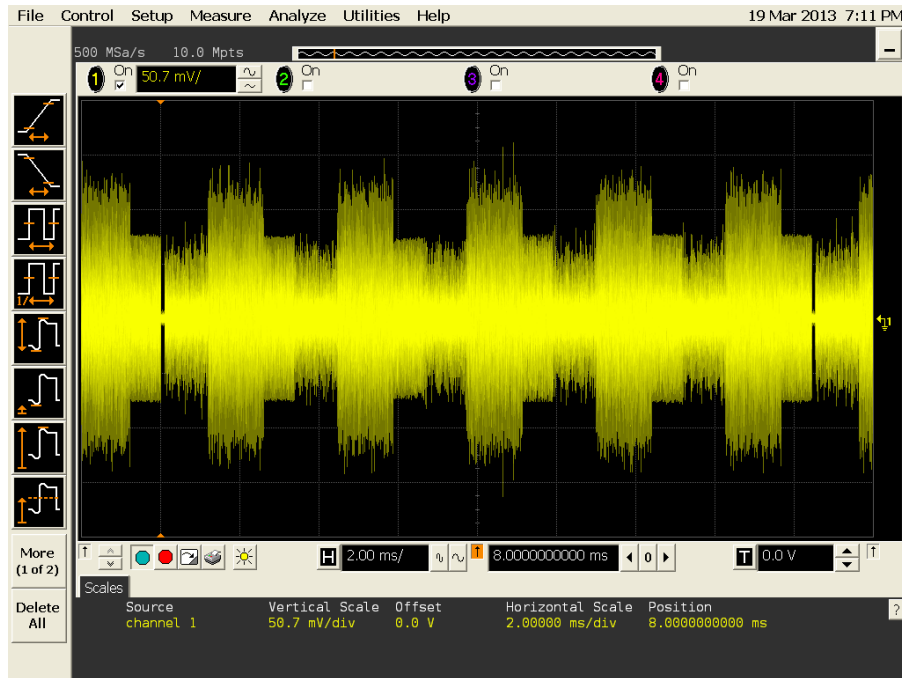
Fig. 7.9: Screen from oscilloscope displaying RF signal with zero gaps.
