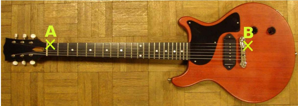
Figure 9.1: One of the 11 guitars of the study. The crosses indicate the measurement points. Point A is close to the nut, on the 1st string's side. Point B is close to the bridge, on the 1st string's side
