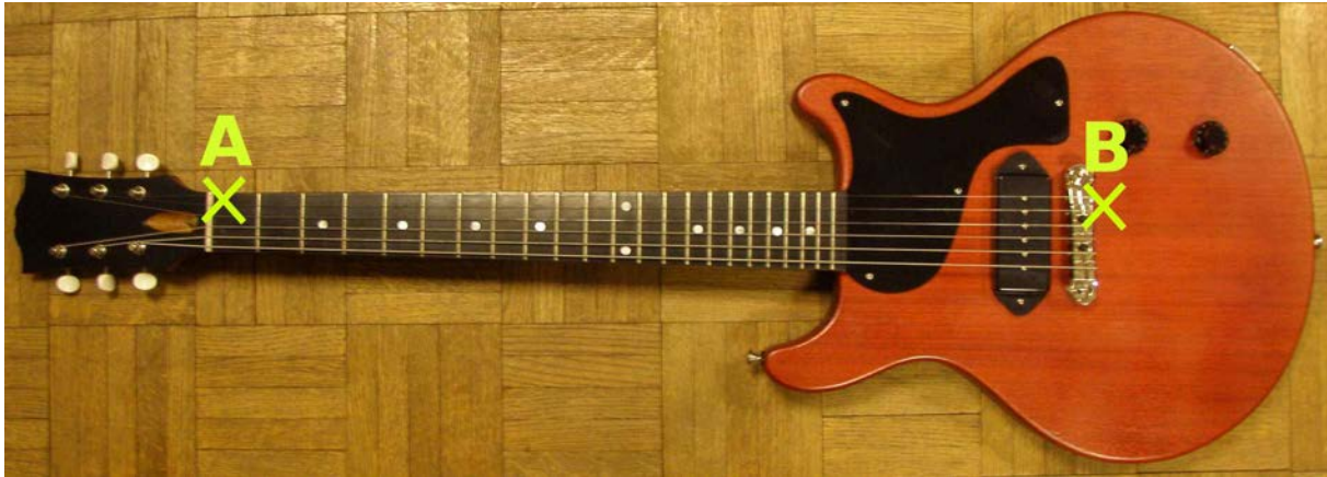
Figure 9.1: One of the 11 guitars of the study. The crosses indicate the measurement points. Point A is close to the nut, on the 1st string's side. Point B is close to the bridge, on the 1st string's side
