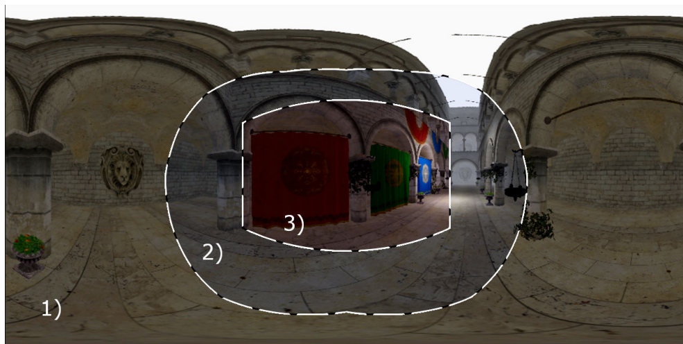
Figure 5.3 – Comparison of the FoV provided by 1) equirectangular projection, 2) human natural binocular vision (light blue), 3) classic perspective projection (light red) with 16:9 aspect ratio ( 75^\circ \times 107.5^\circ ). To maintain consistency, the perspective projection is remapped into the equirectangular projection, making the horizontal limit curved.
