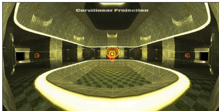
Figure 1.28 – Curvilinear rendering is a PVPE method developed by Oros on the first generation of programmable GPU [Oros 02].
