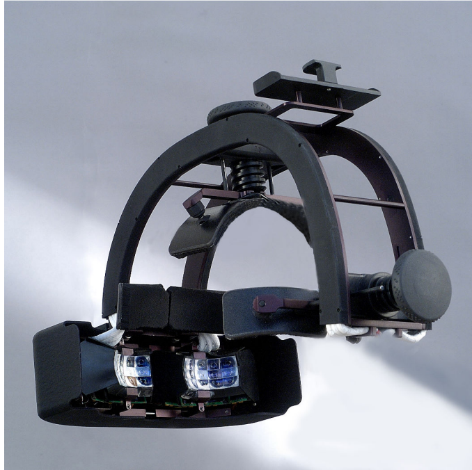
Figure 1.20 – The PiSight HMD from Sensic. Each screen is composed of several OLED matrixes, providing large FoV without sacrificing the definition of the displayed images.
