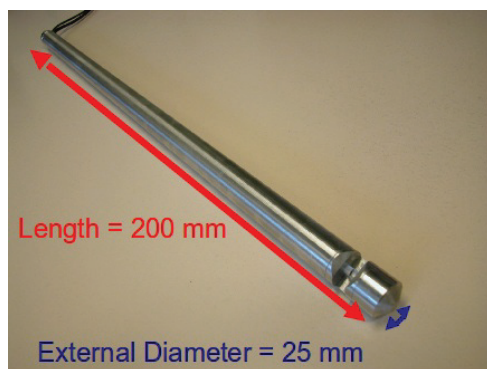
Figure 3.2: Photo and dimensions video probe EZ Probe-D25 L1300, developed at LAGEP
