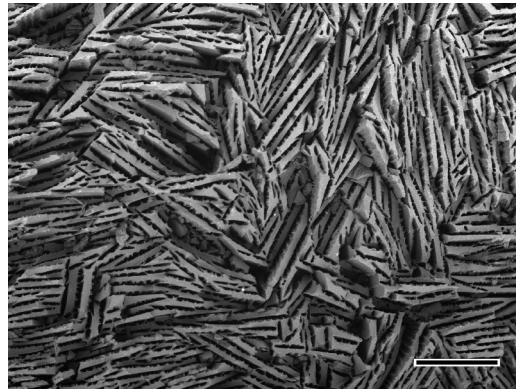
Figure 5.2: Typical porous structure obtained by ice-templating showing the different domains of orientation. Scale bar 0.5 mm.
