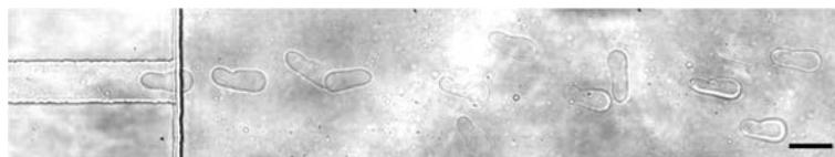
Figure 5.35: Optical micrograph showing that the sol-gel transition can take place so fast that the plug-like droplet becomes solid and can not break into smaller droplets. The continuous phase here is fluorinated oil FC 3283. The scale bar is 20\mu\text{m} .
