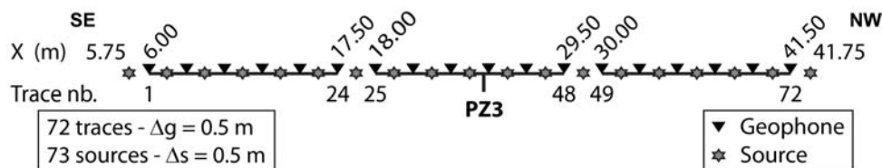
Figure 3.3 : Sketch of the seismic acquisition setup used under both hydrological conditions for combined P-, surface and SH-wave surveys. P- and surface-wave data were obtained using 72 14-Hz vertical geophones, while SH-wave were recorded with 72 14-Hz horizontal geophones. Interval between two geophones ( \Delta g ) and move-up between shots ( \Delta s ) were both 0.5 m. The seismic profile is centred on PZ3. The origin of the x -axis is identical to the one used for ERT (Figure 3.2b).
