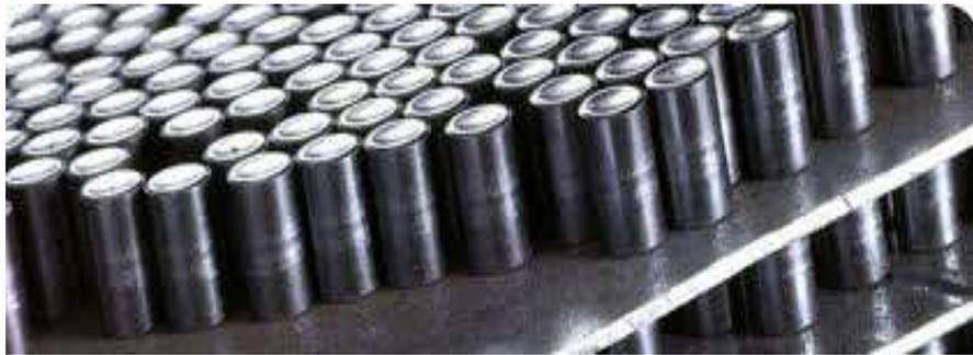
**Figure 2.12.** The pellets of the nuclear fuels.
