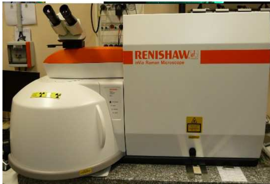
Figure 1.2. InVia Reflex Renishaw Raman system.
