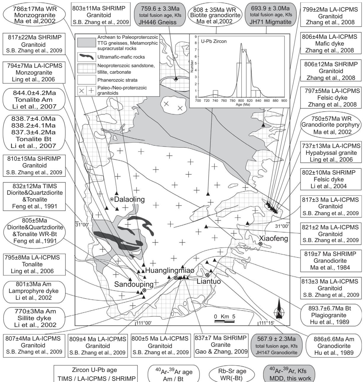
**Fig. 8A.** Compilation of the U-Pb, Rb-Sr and Ar-Ar ages from the Huangling granitoids. Inset statistical chart shows the results of the zircon U-Pb ages. Am, amphibole; Bt, biotite; Kfs, K-feldspar; WR(-Bt), Whole rock(-biotite).
