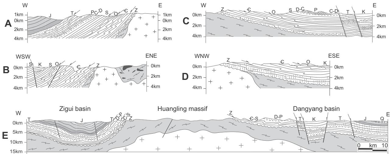
**Fig. 4.** Cross-sections across the Huangling massif (locations in Fig. 2). (A–D) Cross-sections of the western and eastern sides of the massif in different locations. (E) General cross-section traversing the Zigui basin, Huangling massif and Dangyang basin.
