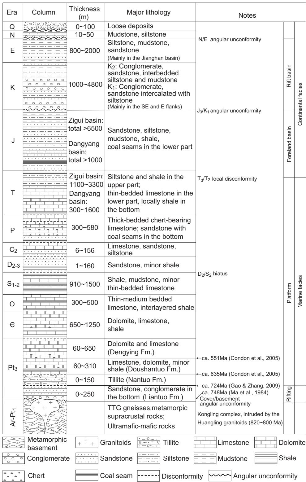
**Fig. 3.** Stratigraphic column of the Huangling area (BGMRHB, 1990). The boundary ages of the Neoproterozoic Liantuo, Nantuo and Doushantuo Formations were dated by zircon U-Pb of volcanic ash or tuff beds (Ma et al., 1984; Condon et al., 2005; Gao and Zhang, 2009).
