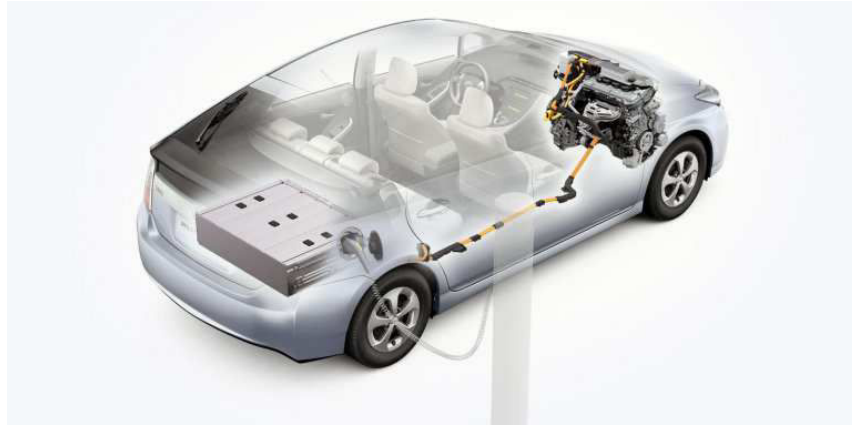
Figure 5-10 Toyota Prius Plug-in Hybrid Electric Powertrain (Beissmann, 2011)
