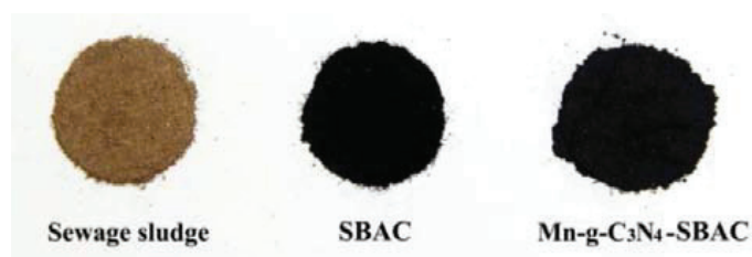
Fig. 4-15. Photos of dry sewage sludge, sludge-based activated carbon and the Mn-g-C 3 N 4 and SBAC composite catalysts.
