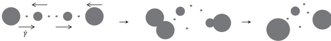
Figure 4.13: Schematic representation of coalescence in the morphology created by end-pinching ( R_v \ll 1 ).
