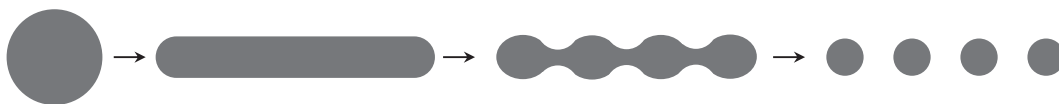
Figure 4.5: Schematic representation of the capillary wave instability mechanism (Rayleigh) leading to drop break-up, that is consistent with the morphology development in uncompatibilized PA6-18k/HDPE blends with a viscosity ratio R_v \simeq 1 .
