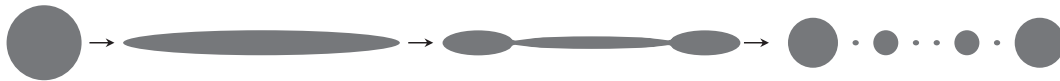
Figure 4.12: Schematic representation of the break-up mechanism by end-pinching and formation of satellites between droplets that is consistent with the morphology development in uncompatibilized PA6-3k/HDPE blends when PA6-3k is dispersed in HDPE matrix with a viscosity ratio R_v \ll 1 .
