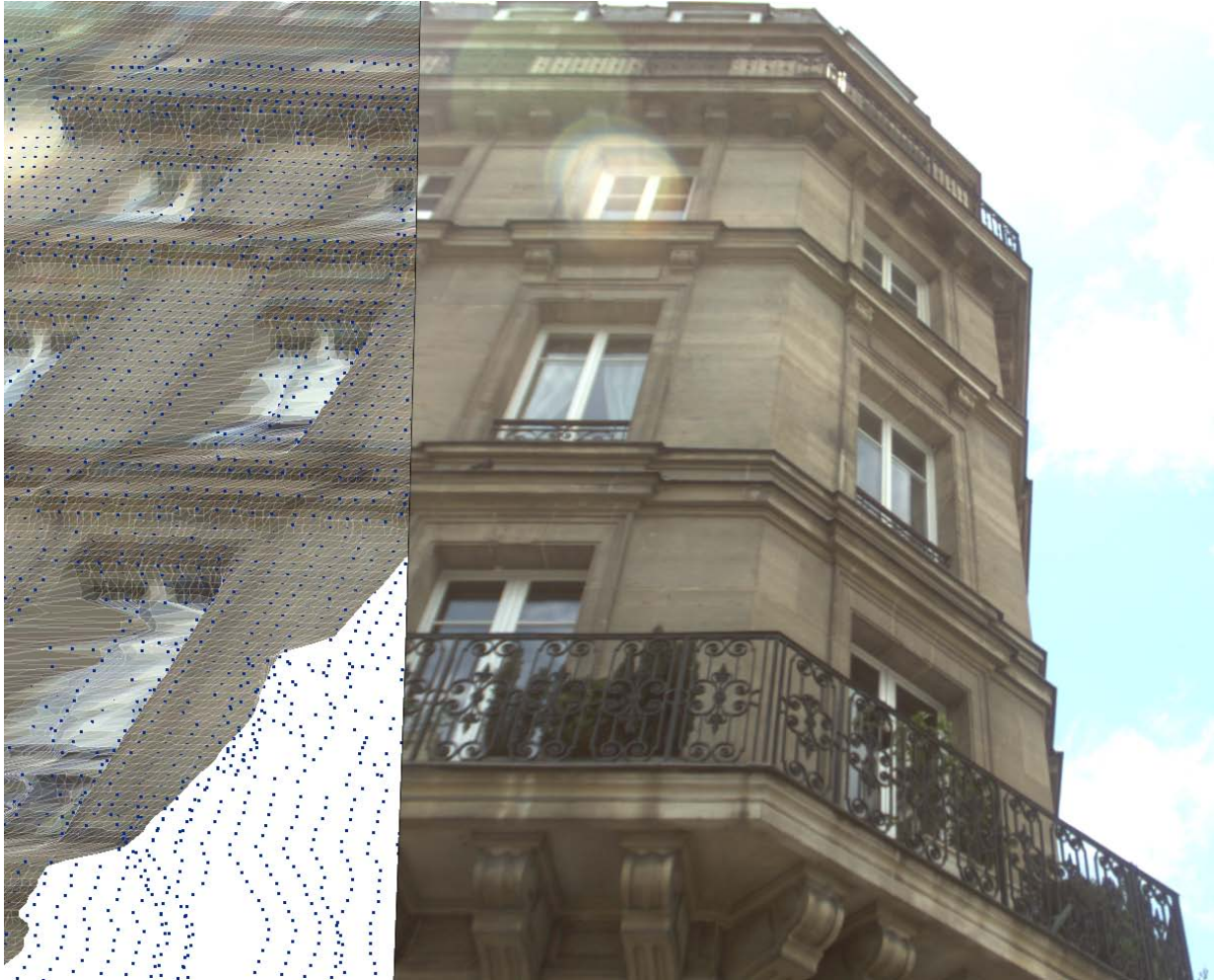
Figure 8.7: Comparison between the textured grid and an image. On the left, the textured grid and the lidar echoes (blue). On the right, an image. The point density is low relative to the image resolution, however, the geometric model is consistent with the texture. The main problems remain at the discontinuities (edges of balconies, window edges). Despite the discontinuity matching algorithm, there are smudges texture. The discontinuities are at the limit of visibility of the lidar sensor and the image sensor. So these are areas that are poorly seen or unseen and where the lack of information needs to be interpolated. This explains the visually imperfect results.
