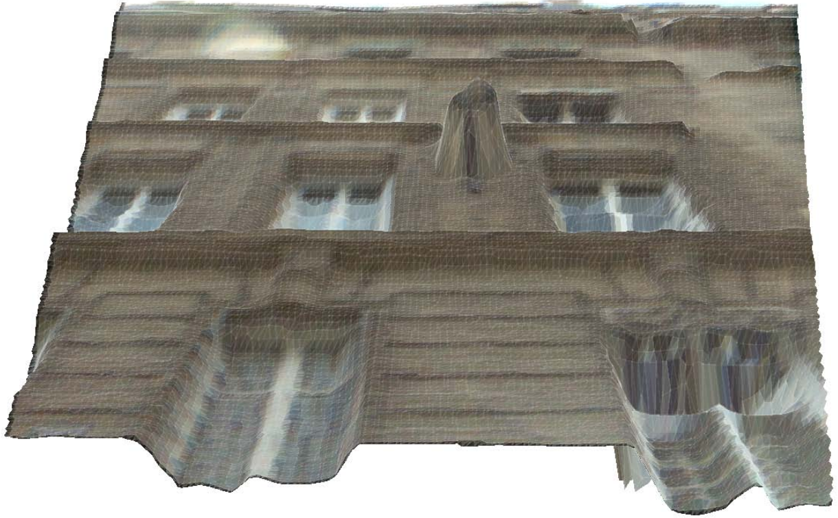
Figure 8.6: Output grid textured with an image. The point of view is close to the sensor point of view, this is the one that showcases the most the result: texture distortions appear all the more we move away from this viewpoint.
