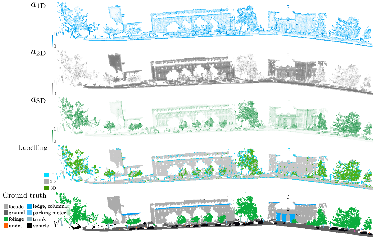
Figure 2.25: Dimensionality features and labellings compared with a manual labeling of the Oakland dataset. One can check visually the consistency between our automatic labeling and many semantic objects such as the ledges and columns (1D), the facades (2D) and the foliage (3D).
