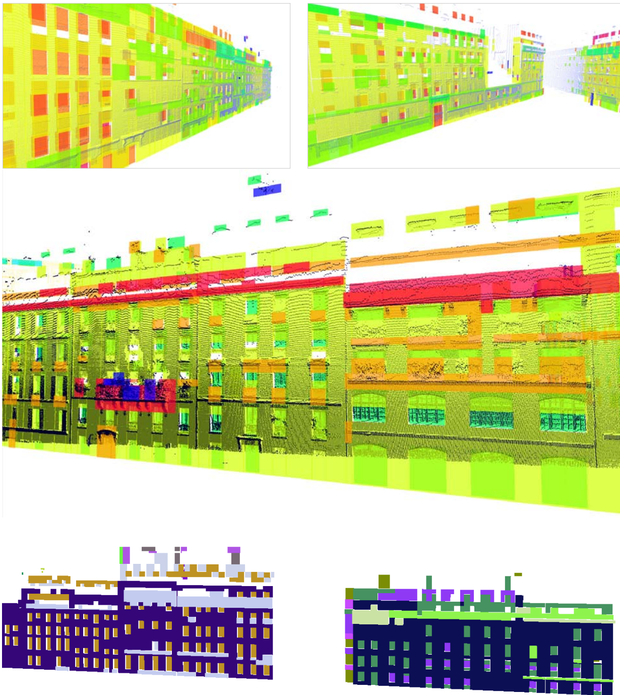
Figure 5.6: Depth Discretization. Only the grid boxes that contain enough points are displayed. The boxes are colored according to their depth values. We do not always understand the meaning of the boxes that do not necessarily correspond to a clearly identifiable object such as a window or balcony. In addition, all windows have no associated box. Indeed, shuttered windows have the same depth as the wall and are therefore not highlighted by a differently colored box. However, boxes highlight the overall structure of the facade. One can observe specific behaviors on each floor, such as the first floor balconies, and one can see that the box sizes and positions vary between buildings of the same alignment. Boxes could therefore provide clues for understanding the facade grammar.
