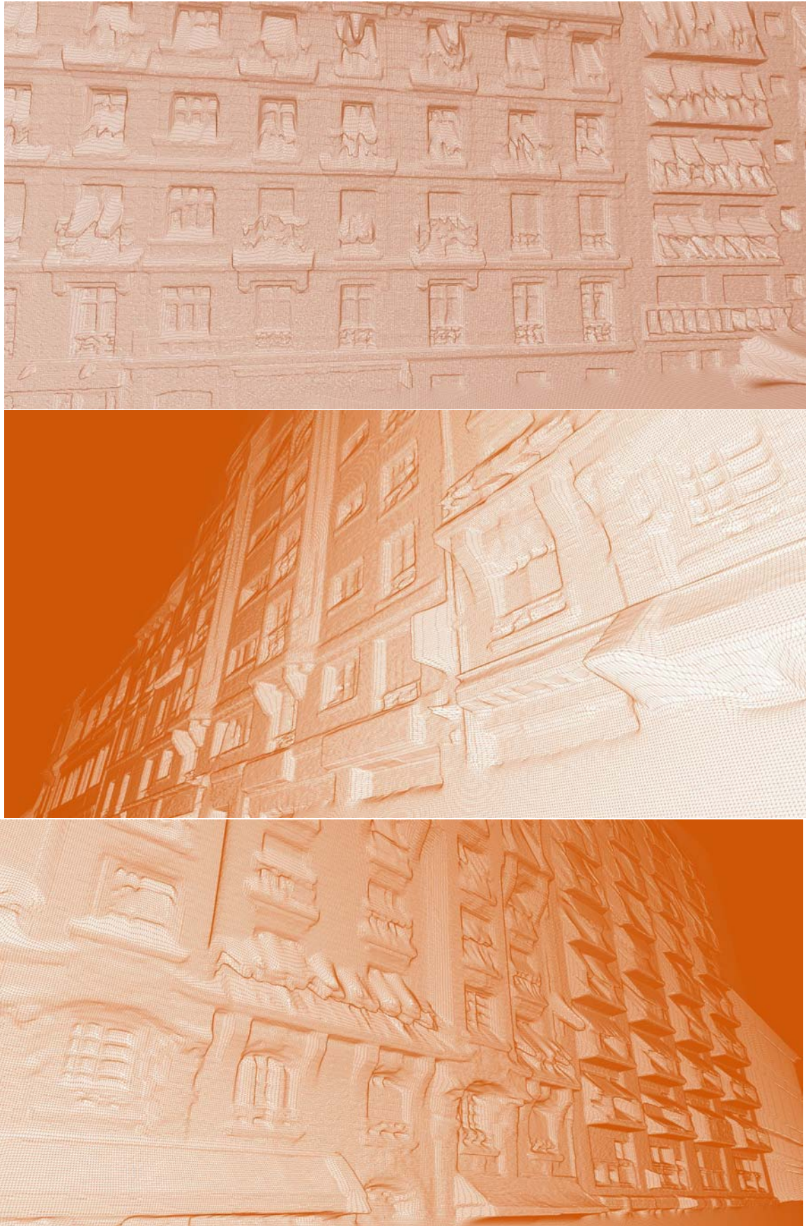
Figure 7.18: Some results on a facade with complex architectural patterns. Shapes are well approximated thanks to the deformable grid (Prismatic coordinate system). However, the model gives an impression of material that is melting or flowing down. This is because the surface covers all hidden areas that can actually be empty. However, with this single street point of view, it is impossible to know if such areas are empty or full.
