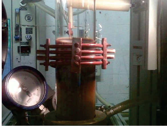
Figure II.20: State of the reactor after several growths with Ge (deposit on the side walls)
