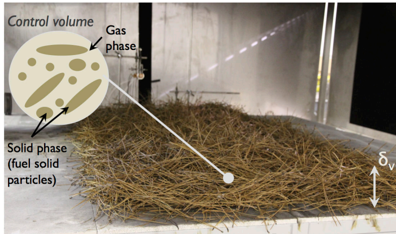
Figure 3.2: Vegetation of thickness \delta_v (5-10 cm) made of pine needles (solid fuel particles or solid phase) and a gas phase.
