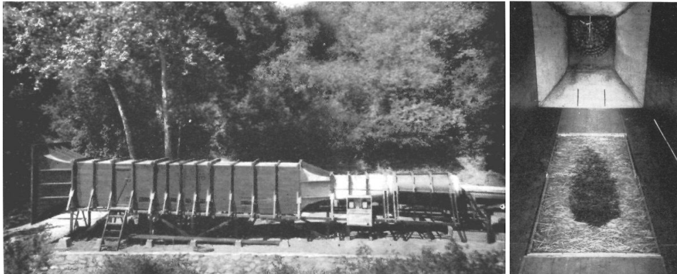
Figure A.1: Wind-tunnel experiments of fire spread: the test section is 9.2 m long with a cross section of 1.8 m \times 1.8 m and pine needles are used to model typical Californian vegetations. Credit: Fons (1946), US Forest Service.
