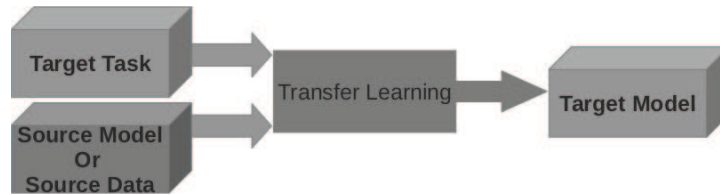
Figure 2.7: Transfer learning. Is machine learning with an additional source of information apart from the standard training data, i.e., knowledge from one or more related tasks.
