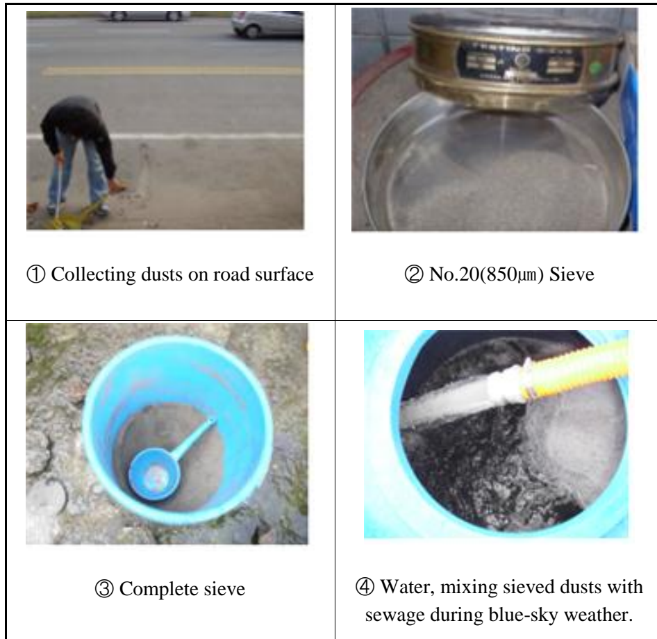
Figure 3.3 Manufacturing process of test samples from NPS pollution
