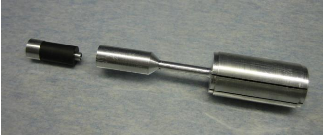
Fig. 4. Initial assembly of the graphite sample (in black) inside the cell (in grey) in the second mock-up
