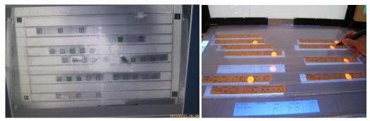
Figure 41: Strip tracking system with bottom and top projection.
