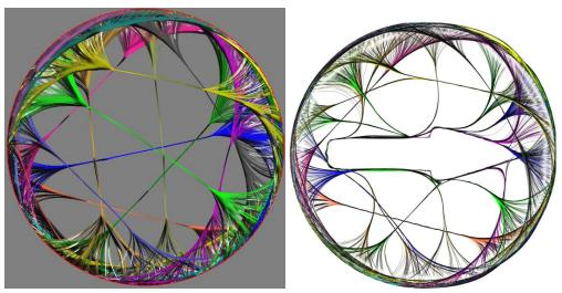
Figure 30: Bundling of dependency graph with obstacle ovoidance (right).
