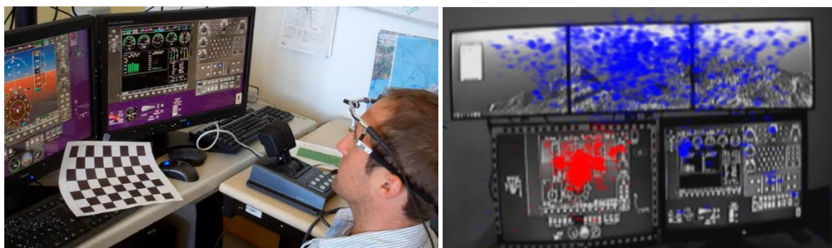
Figure 51: Simulation environment with head mounted eye tracking system (left). Visualization of fixation points inside the cockpit when gathering flight parameters in red, and elsewhere in blue.
