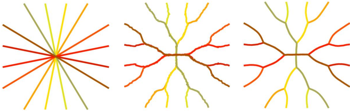
Figure 43: Raster map size effects. Original graph (left), bundled version with a small raster map (middle) and with a large raster map (right).
