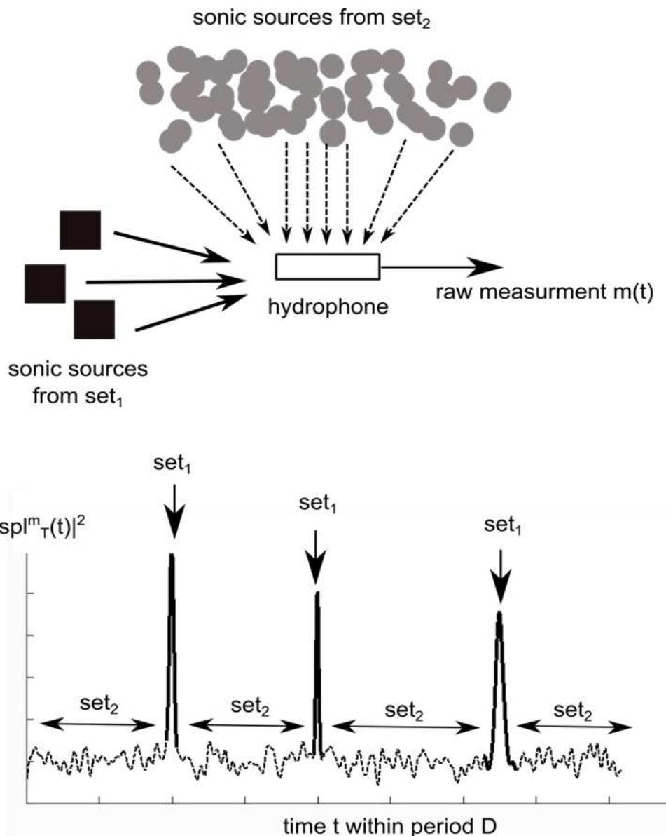
Figure 2.4: Ocean noise (marine soundscape measurement) consisting of occasional loud transient (set<sub>2</sub>) overlaying the background noise (set<sub>1</sub>) [Gervaise13]
