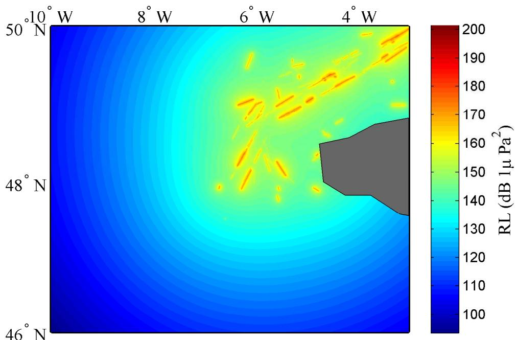
Figure A.7: Spatial distribution of cumulative hourly shipping noise in Ushant, from simulation using RANDI spectra and the ship position from AIS. The received level was computed in the 1/3 octave around 65 Hz
