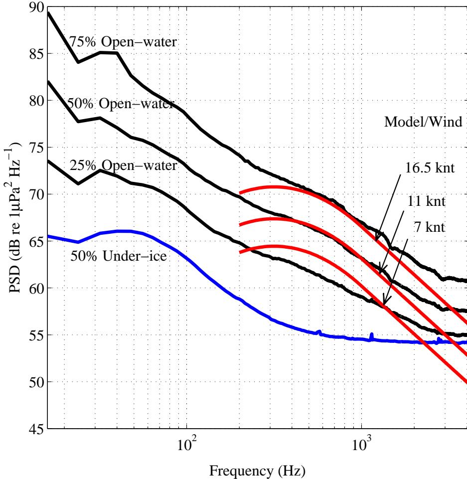
Figure 4.9: Open-water ( $\pm 1$  quartile) ambient noise spectra and under-ice median spectrum in the Beaufort Sea. Modeled wind-generated ambient noise in the 200-4000 Hz bandwidth are given for the 25<sup>th</sup>, 50<sup>th</sup> and 75<sup>th</sup> percentiles of open-water period winds in the Amundsen Gulf mouth.
