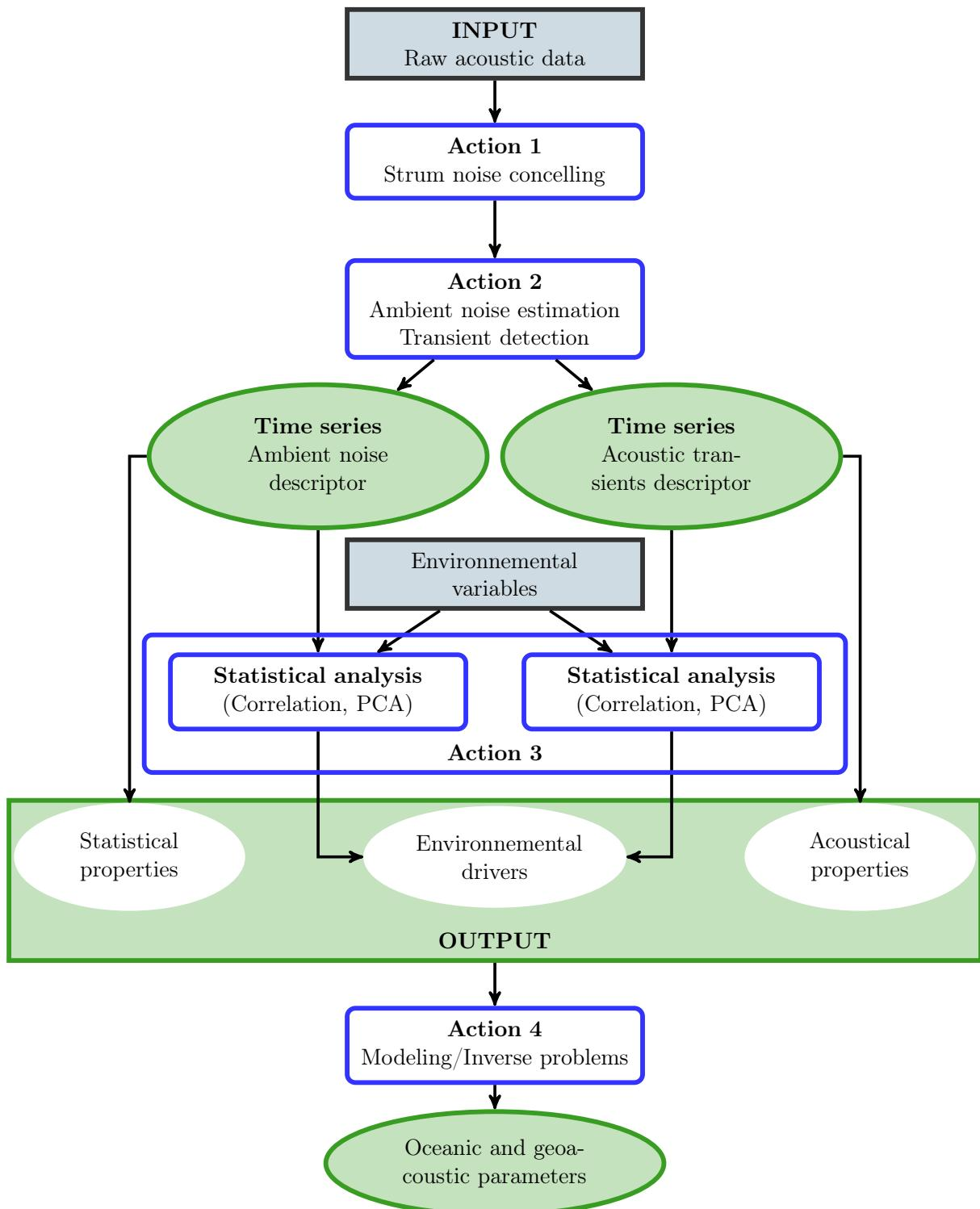
Figure 2.6: Conceptual diagram of passive acoustic monitoring processing.
