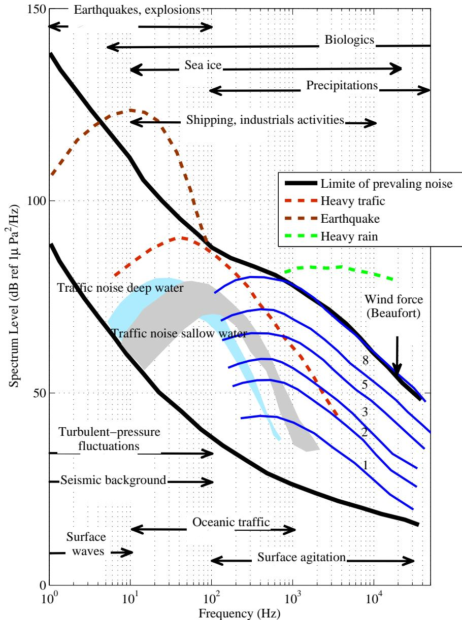
Figure 2.5: Wenz Ambient noise spectra [Wenz62], showing the different contributions to the ambient noise in the ocean. The infrasonic zone is dominated by surface wave, the low frequency by the shipping noise and the low to high frequency by surface agitation. Some occasional sound can dominate locally the ambient noise spectra.
