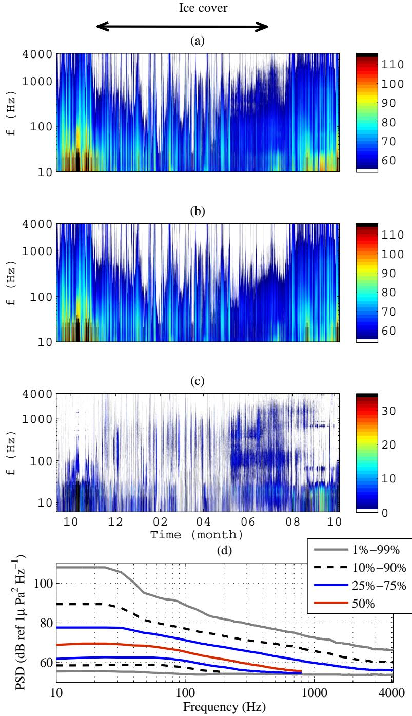
Figure 4.13: Annual spectrograms of the recordings in the Amundsen Gulf showing, (a) the total ocean noise hourly spectral levels; (b) ANL hourly spectral levels; (c) their ratio; and (d) the ANL percentiles. White pixels correspond to bins with levels below the instrument self noise in (a) and (b) and to a ratio of 1 (0 dB) in (c).
