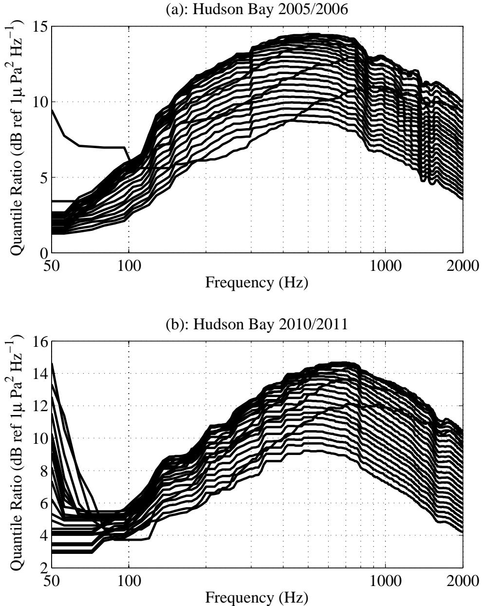
Figure 4.11: Ratio open-water/under-ice ambient noise spectra for percentiles  $\geq 50\%$  in the Southeastern Hudson Bay for 2005–2006 (a) and 2010–2011 (b).
