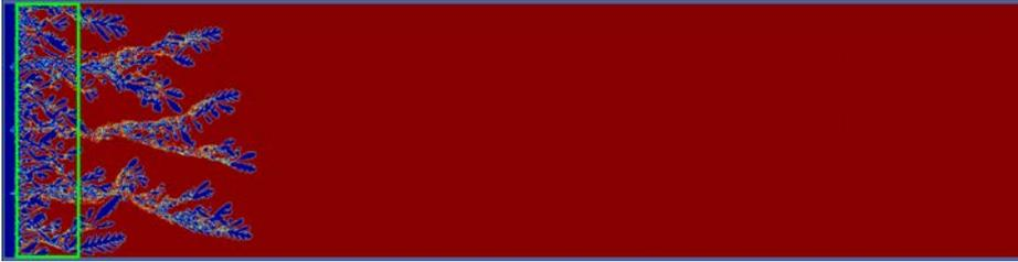
Figure 4.21: Waterflooding simulation. Inside the green rectangle, the oil is not mobilised by any polymer solution.
