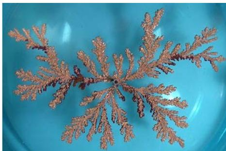
Figure B.3: A DLA-like cluster obtained by diffusive growth from a copper sulfate solution in an electrodeposition cell. [433]
