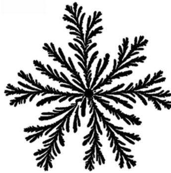
Figure 1.23: Fingering pattern realised in a Hele-Shaw cell (cluster diameter 200 mm). [198]
