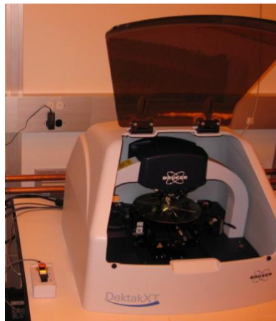
Figure Appendix-36: The Bruker Dektak XT profilometer.
